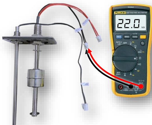
Figure 41 – WLS-L Resistance
