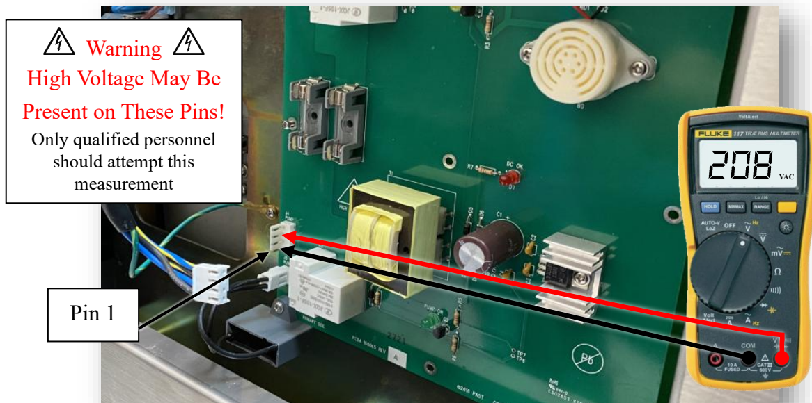
Figure 24 – Pins 1 and 3 (Pump Motor Winding Input Voltage)
