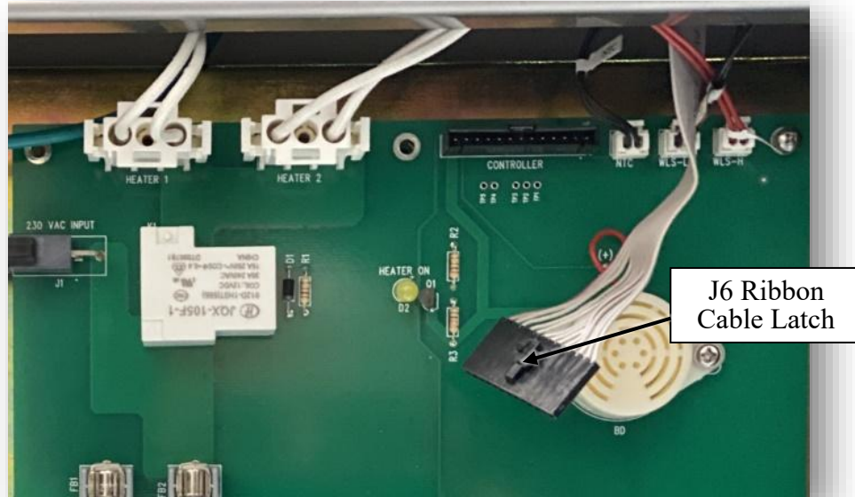
Figure 20 – J6 Ribbon Cable
